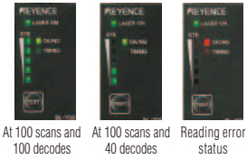
Stable reading indicator using bar LEDs
